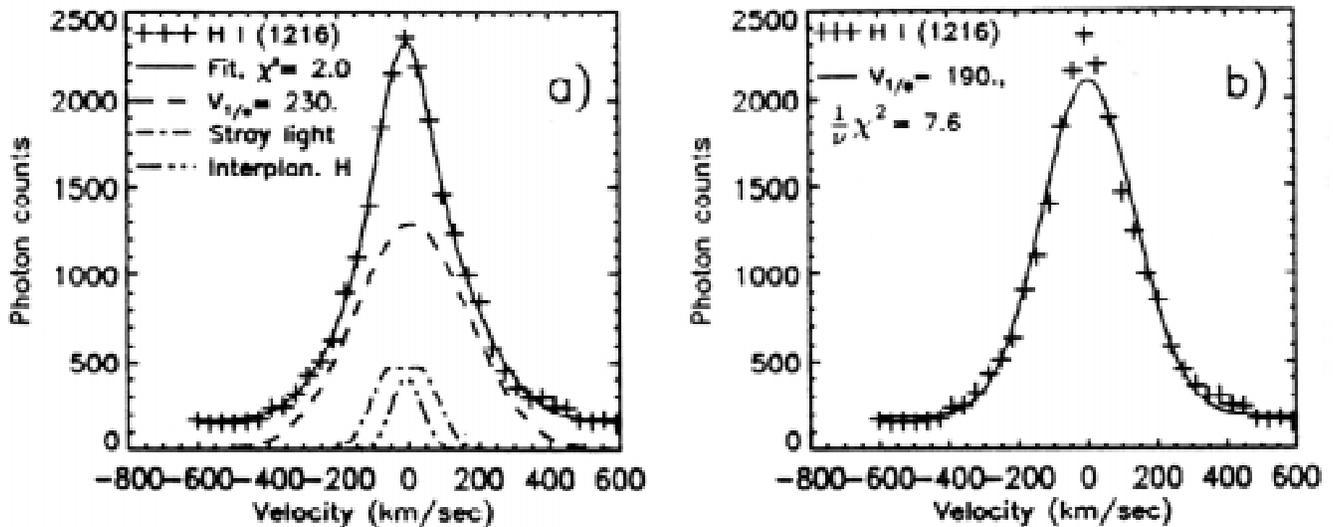
**Figure 10.** HI Ly $\alpha$  profiles for the south polar coronal hole at  $3.0 R_S$  observed on 11 May 1996 from SOHO/UVCS. Computer fits for a single Gaussian plus a constant (b) and three Gaussians plus a constant (a) are shown. The narrow component corresponds to a kinetic temperature of  $O[10^6]$  K ( $v_{1/e} \sim 130$  km/s). The broad component corresponds to  $v_{1/e} \sim 240$  km/s and includes the effects of both thermal and nonthermal motions (Kohl et al., 1997).
