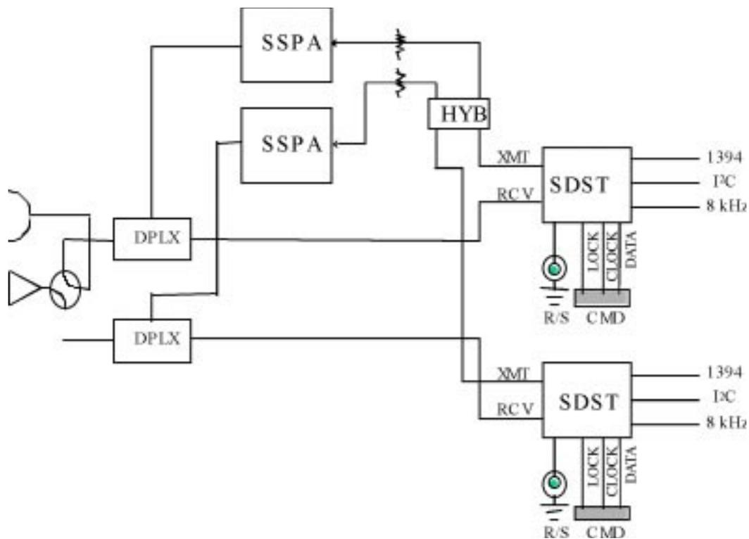
**Figure 23.** Telecommunications subsystem architecture. (CMD = command; DPLX = diplexer; HYB = hybrid device; R/S = Reed–Solomon coder; RCV = Receive; SSPA = solid-state power amplifier; SDST = small deep-space transponder; XMT = transmit.)
