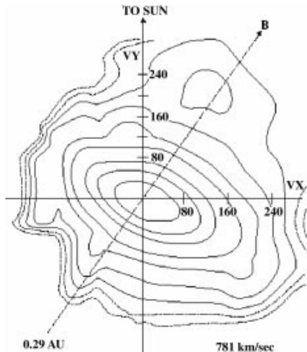
**Figure 5.** Contours of solar wind proton velocity distribution in fast wind at 0.29 AU measured by Helios. Contours are 0.8, 0.6, 0.4, 0.2, 0.1, 0.03, 0.01, 0.003 and 0.001 of the maximum phase space density. The distribution is anisotropic ( $T_{\text{perp}} > T_{\text{parallel}}$ ), hot, and has a faster component along the magnetic field direction (dashed line) (Marsch et al., 1982).
