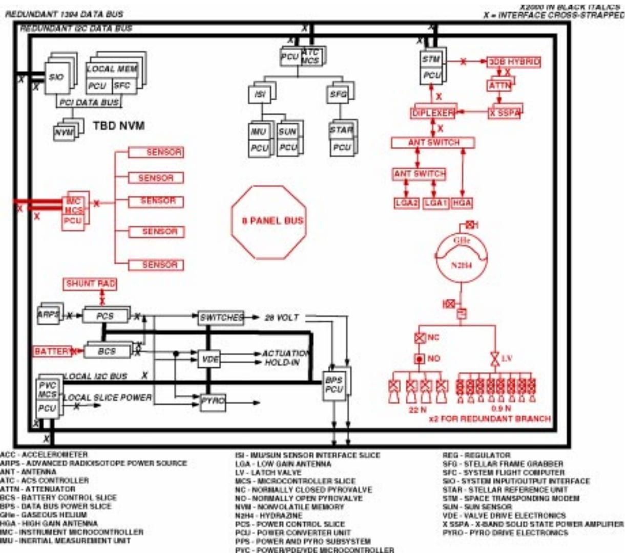
Figure 20. Functional block diagram of the Solar Probe.
